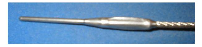
NOT AFFECTED: Flat swaged or crimped pin.
